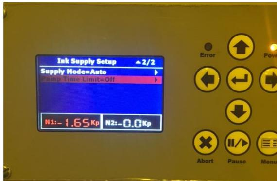
11. Re-enter Pump Time Limit setting menu, and change time limit back to 30 seconds.
