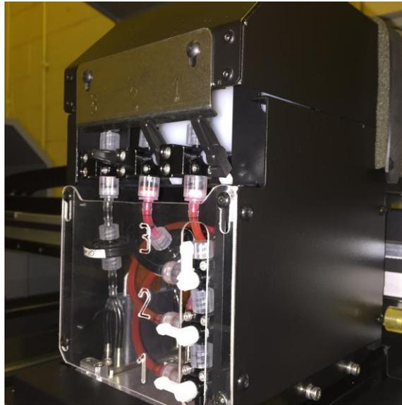
13. Once valve positions are verified, hold 'F' button until all connected tubing to printhead is full of the pink flushing solution.
