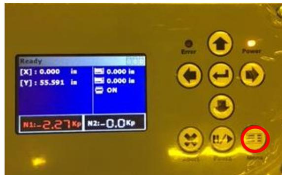
2. Press down arrow until 'Ink Supply Setup' option is highlighted, then press right arrow to advance.
