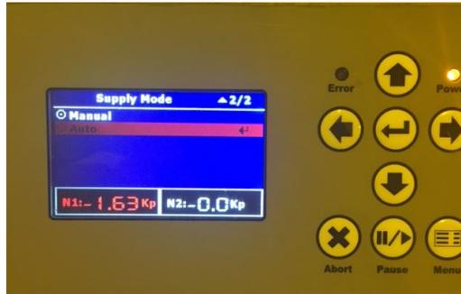
5. Now press "Menu" button, to get back to original screen to verify that alarm is dismissed. Once verified redo steps 1 and 2, to enter "Ink Supply Setup" page.
